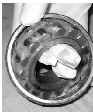
Fig. 21. Grease can easily be packed by hand.
