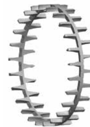
Fig. 45. One-piece, machined-brass, land-riding, finger-type cage.
