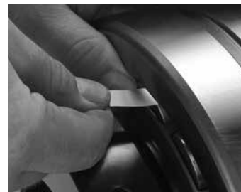
Fig. 97. Measure of RIC before installation.
