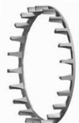
Fig. 46. Split, machined-brass, land-riding, finger-type cage.
