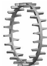
Fig. 44. One-piece, machined-brass, roller-riding, finger-type cage.
