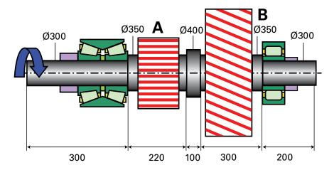
This is an example of an application that can be analyzed in SYBER Bearing System Designer. This sample application shows a two-row tapered roller bearing (TDO) in the fixed positions and a single-row cylindrical roller bearing (NU-style) in the float position on a shaft with different gear types.
