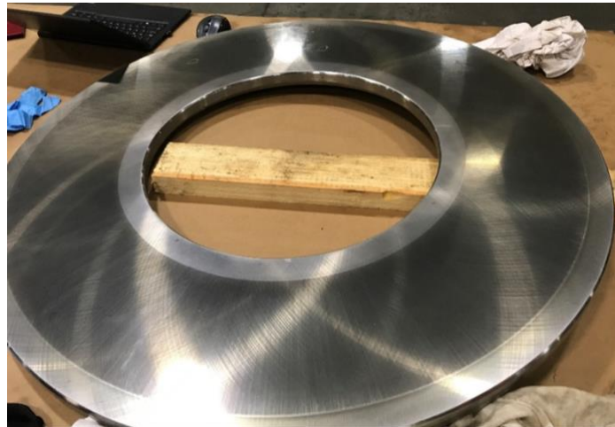
Figure 6: DuraSpexx® Power Rating Series TTHDFL flat thrust race from 1250-ton top drive after a five-year campaign.
