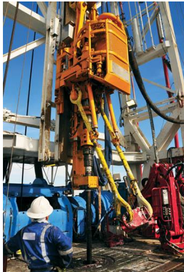
Figure 1: Oilfield top drive, with integrated motor and transmission, hangs from the traveling block and hook in the mast. The motor turns the drill stem and bit downhole.
