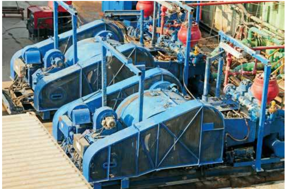
Mud pumps are single-acting or double-acting designs. These design differences are a factor in bearing performance.
