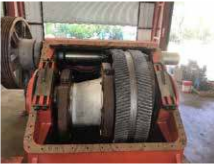
Figure 6: View of installed crankshaft assembly with rear cover removed.
