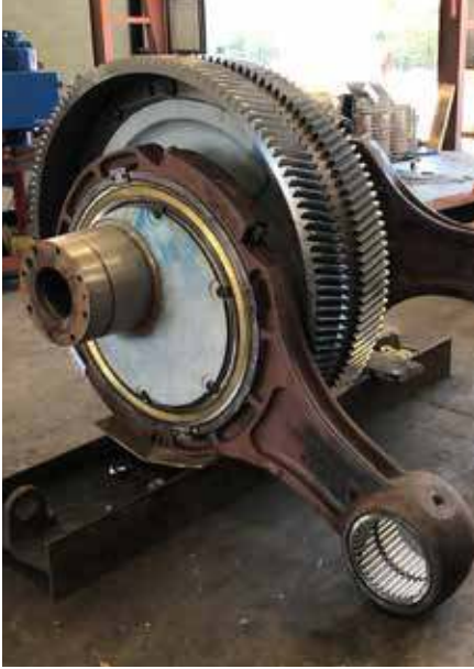
Figure 2: Crankshaft with connecting rods, eccentric, and crosshead bearings before main bearing installation.
