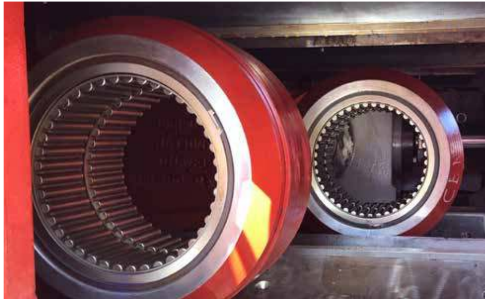
Pictured are Timken right and center crosshead wrist pin bearings. Bearings were used in mud pumps.
