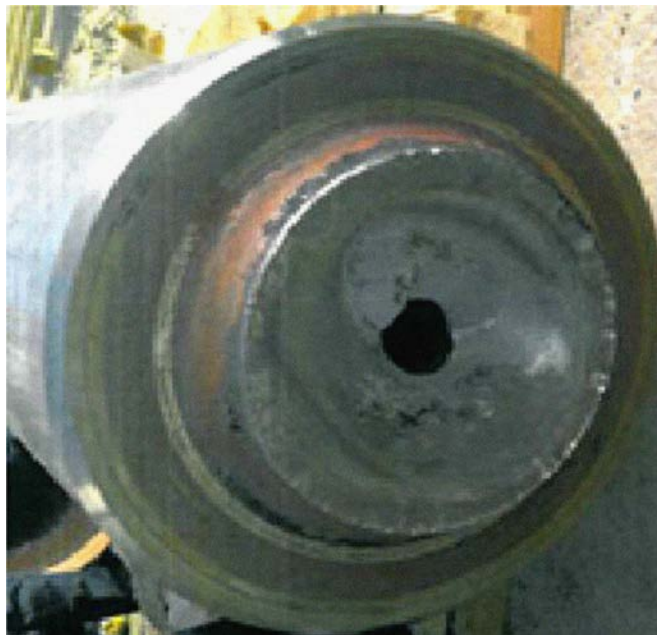
Figure 12: Roll neck breakage.
