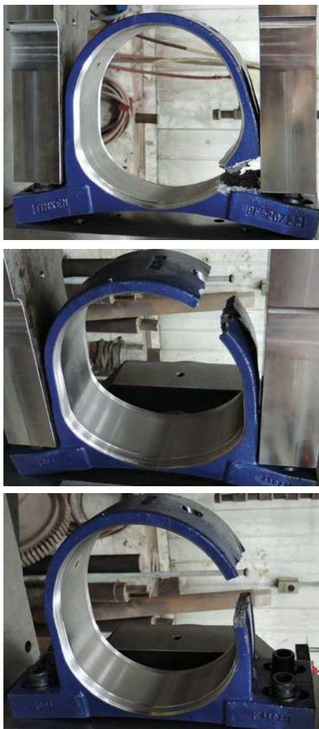
Figure 4: Fracture of split housings.
