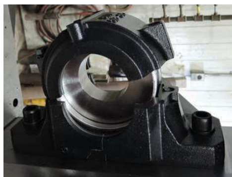
Figure 6: Fracture of split housings.
