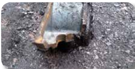
Fractured competitor housing led to unplanned replacement of housed unit.
