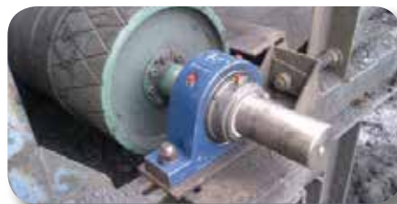
Timken solid-block spherical roller bearing housed unit steps in to meet the challenge.
