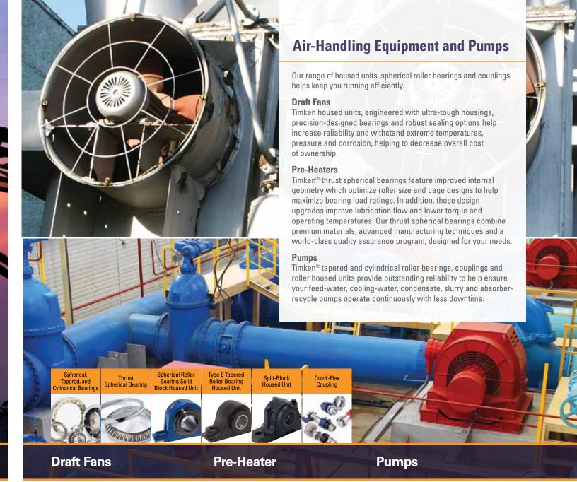
Timken roller bearing housed units, available in a large range of customary and metric sizes, feature precision-engineered Timken bearings, durable housings, multiple sealing options and housing covers best suited for the task. These units are an excellent choice for induced-draft and forced-draft fans.
