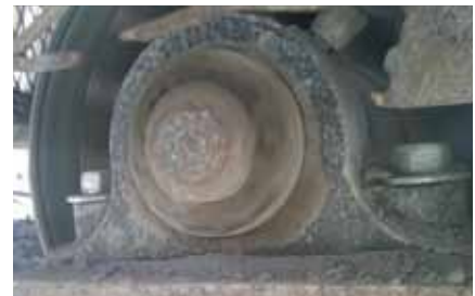
Conveyors at Boxley's aggregate quarry mill now run on Timken Type E tapered roller bearing housed units, resulting in greater uptime and reliability.
