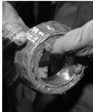
Fig. 149. Grease can easily be packed by hand.
