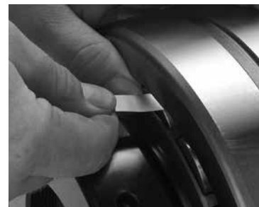
Fig. 95. Measure RIC before installation.
