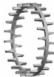
Fig. 44. One-piece, machined-brass, roller-riding, finger-type cage.
