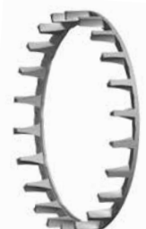
Fig. 46. Split, machined-brass, land-riding, finger-type cage.
