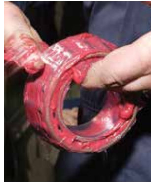
Fig. 58. Grease can easily be packed by hand.
