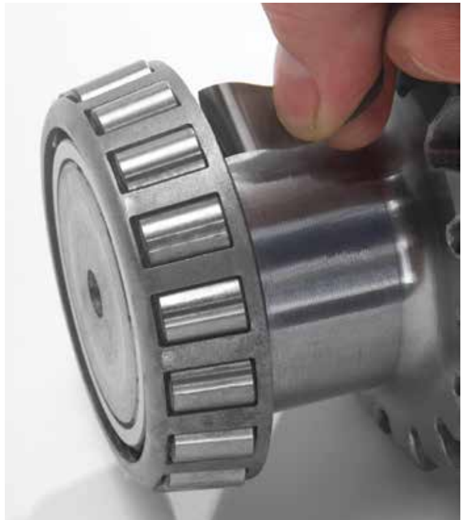
Fig. 23. Bearings should be checked with a feeler gage to ensure proper fit.
