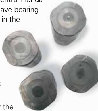
Bearings after 6 months of operation
