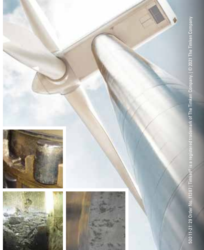
Pictured above is damage seen in the field on spherical roller bearings used in three-point mount turbines.
